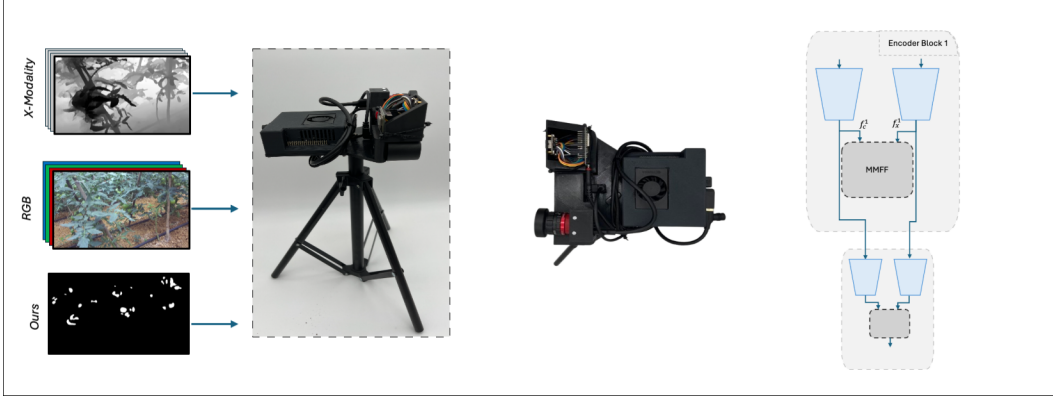
Figure 2: Our multimodal handheld data acquisition platform. The device integrates a ZED 2i stereo camera for RGB, depth, and pose; an Allied Vision NIR camera; and a Teledyne FLIR thermal camera. All components are mounted on a rigid frame with an onboard Jetson Orin Nano for synchronized capture and storage..
